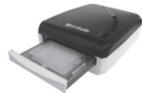
(C) Record the activity of the plate with worms using wMicrotracker ONE
